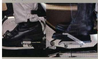
The Cavalcade LX sports adjustable co-rider footboards to help resist leg and upper thigh fatigue. Rider footpegs can be pre-set to any one of three convenient positions.
