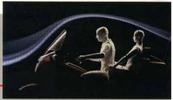
The design of the LX's fairing/windshield helps shield riders from rain at cruising speeds and minimizes wind noise. Fairing vents allow rider to use engine heat in cold weather.
