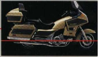
Suzuki's pneumatically-controlled "Auto-Levelling System" provides automatic adjustment of vehicle's ride height to compensate for variations in vehicle payload.
