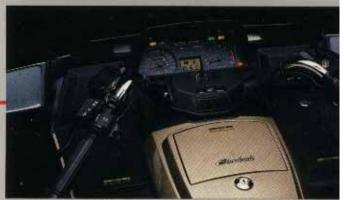
The fully-instrumented cockpit informs you of most major mechanical functions. Note the handlebar-mounted controls for the stereo, cruise control and optional intercom and CB.
