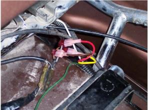
Figure 3 – t-tap attached to the right saddlebag wire
