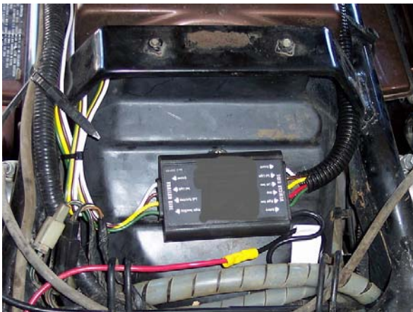
Figure 1 – mount the adapter to the inner fender under the seat
