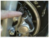
1) Disconnect the lower front lines from the calipers at the swivel joint and remove the swivel adapter from the caliper.
