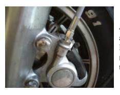
4) Thread the swivel nut on the lower end of the line onto the adapter fitting installed into the caliper on step 2. You can turn the line so that it's natural curve fits it's location. Tighten the swivel nuts on both ends of the line (7/16" wrench). Since they seal on a taper, they need to be good and snug but not overly tight.
